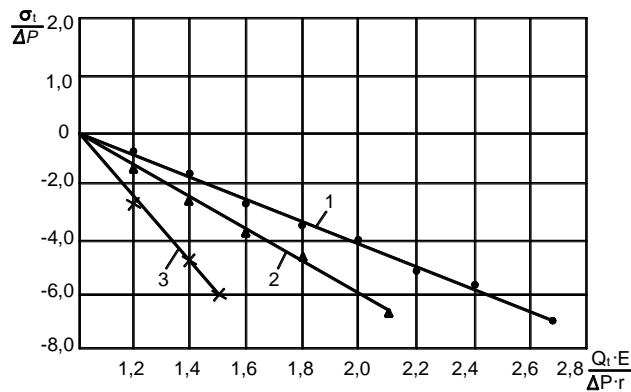
Fig. 13. The dependence of the axial tension on the tightening force: 1-×; 2-▲; 3-●;
