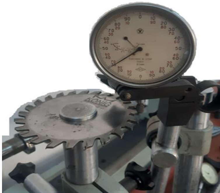
Fig.1. Device for measuring the deformation of the teeth of a disc cutter
