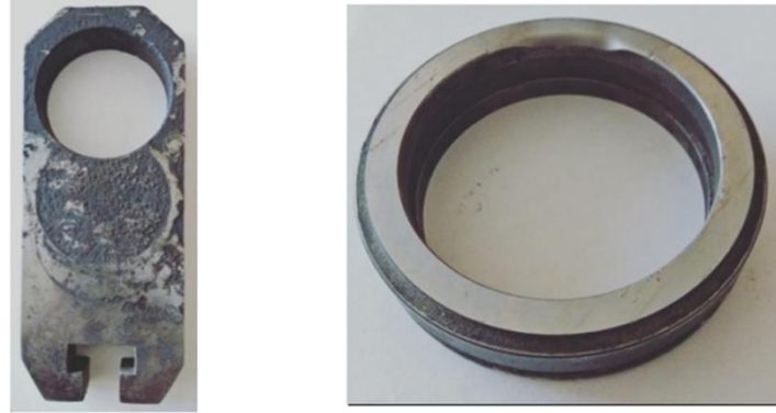
Fig. 2 Common malfunctions during the operation of a knife gate valve at an oil field
